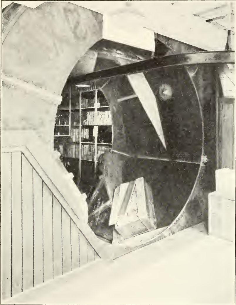
Large revolving hexagonal drum box-testing machine. Dimensions, 14 feet inside diameter and 8 feet in width
